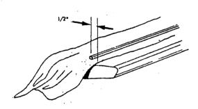
C. For side pockets, start approximately 3" from end of rail and pull cloth toward rubber cushion until the edge of the cloth is approximately ½" from the end of the feather strip. Tap feather strip in place.
